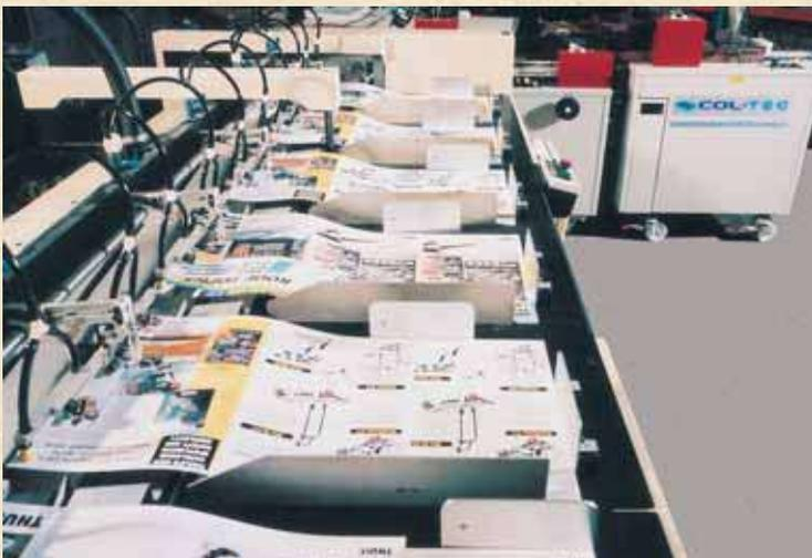
Refurbished 6 station SRA3 collator and stitch/fold/trim line installed at customers premises, overall dimensions 390 x 110 cms
